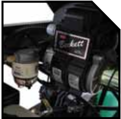
12 Volt Burner with fuel/water separator
